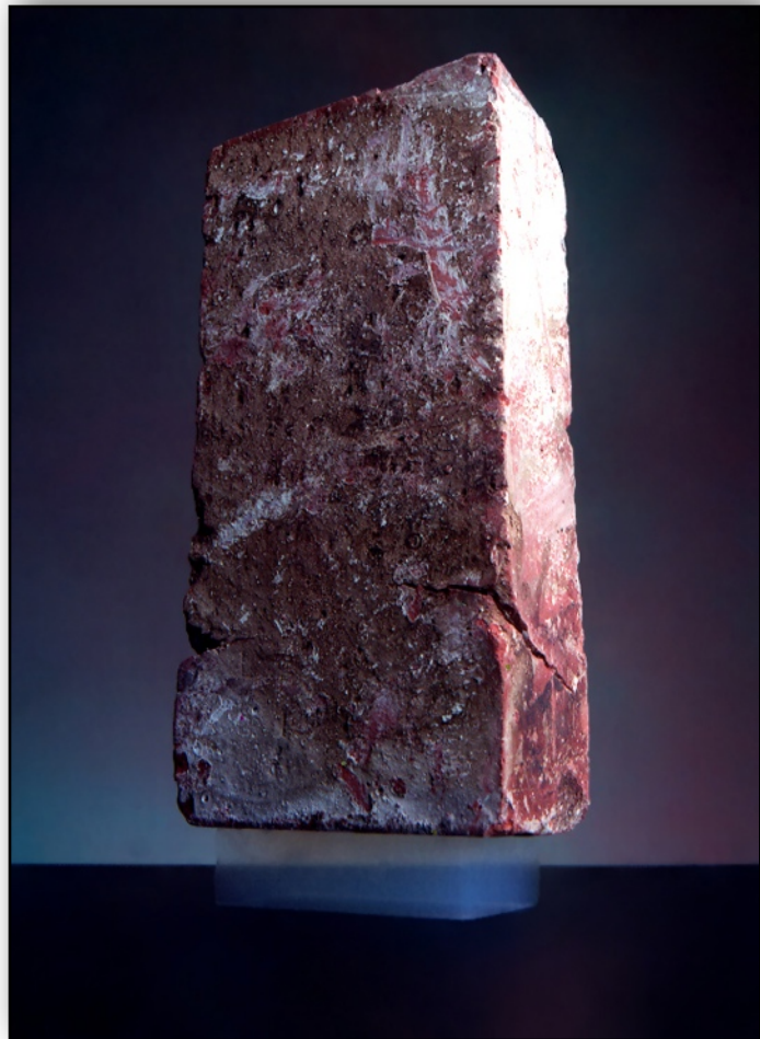
Figure 8: A 2.5 kg brick is held up by a piece of aerogel weighing only 2.38 grams. Aerogel is a low-density material derived from gel impregnated with gas. The result is an extremely low density solid with several remarkable properties, most notably its effectiveness as a thermal insulator and strength. Aerogel is able to hold over 2000 times its own weight (see: NASA ).
