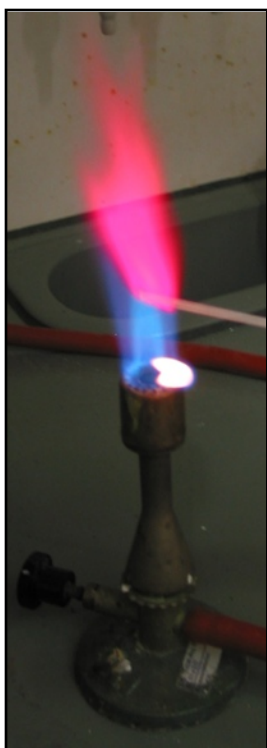
Figure 6: Lithium burns with a bright red glow. During the expedition to the Salar de Uyuni the i2P team will be enriching and burning lithium.
